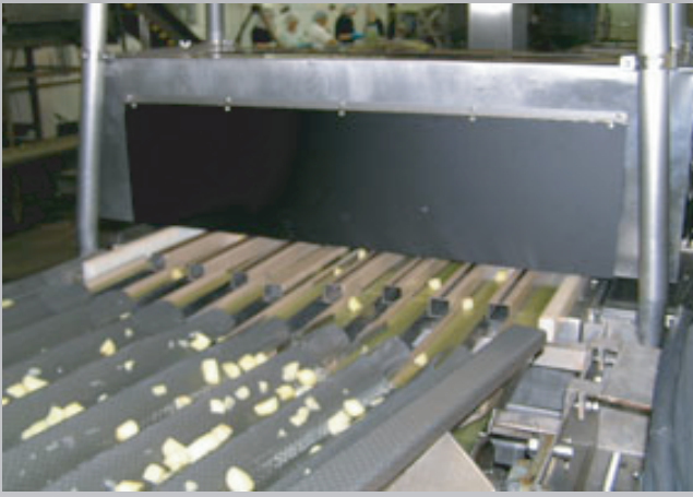
Ginger pieces on vibratory feeder, being fed onto scanning conveyor belts
