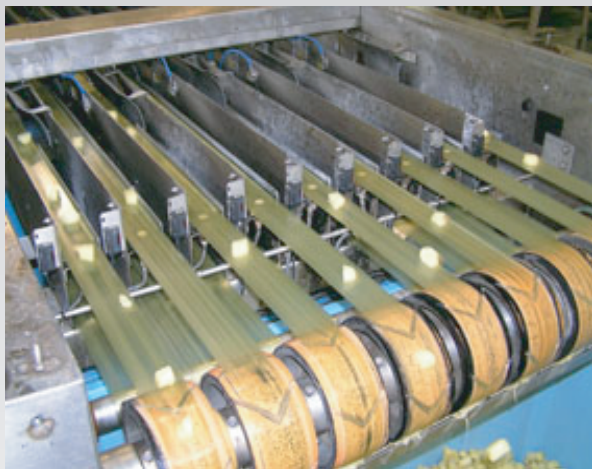
Pieces going into last sort bin. This existing conveyor and vibratory feed system was re-used with the all new control and scanning system. A complete new system could however be provided including all the product handling.
